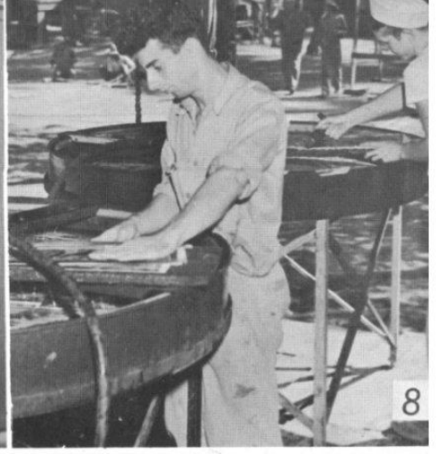
(1) The Photo-Lab installation in the Philippines. (2) Sgt. Green recording a mission on the mission board. Information on missions was telephoned from operations. (3 & 4) Developer, hypo or short stop being mixed by Cpl. Schmitz. (5 & 8) Prints were first washed in a sink to remove excess hypo, then washed in the regular washers. Cpl. Roemer and Pvt. Smith are using the sink. Sgt. Drake and Cpl. Petrillac are doing the final washing. (6) Sgt. Lyon has just finished developing a film (7) Sgt. Peterson drying the film after it had been washed. (9) The negatives were lettered after the Intelligence officer selected those to be printed. Cpls. Konupek, Esmond and Sgt. Fiori are shown engaged in their work.
