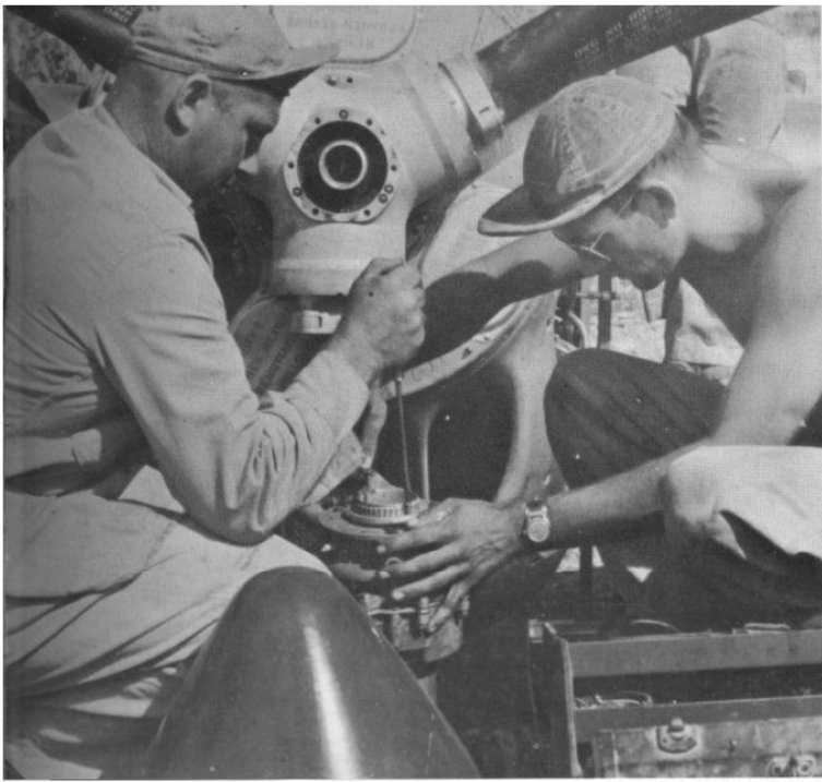
(Top) All the propeller work was done by Sgt. Kammerer and Cpl. Hachman. In the picture, they are working on the electrical contact points in the prop motor which change the pitch of the propeller to effect a constant engine RPM. (Bottom) Our only hydraulic specialist was Sgt. Coker. He is shown installing a multiple disc brake unit.
