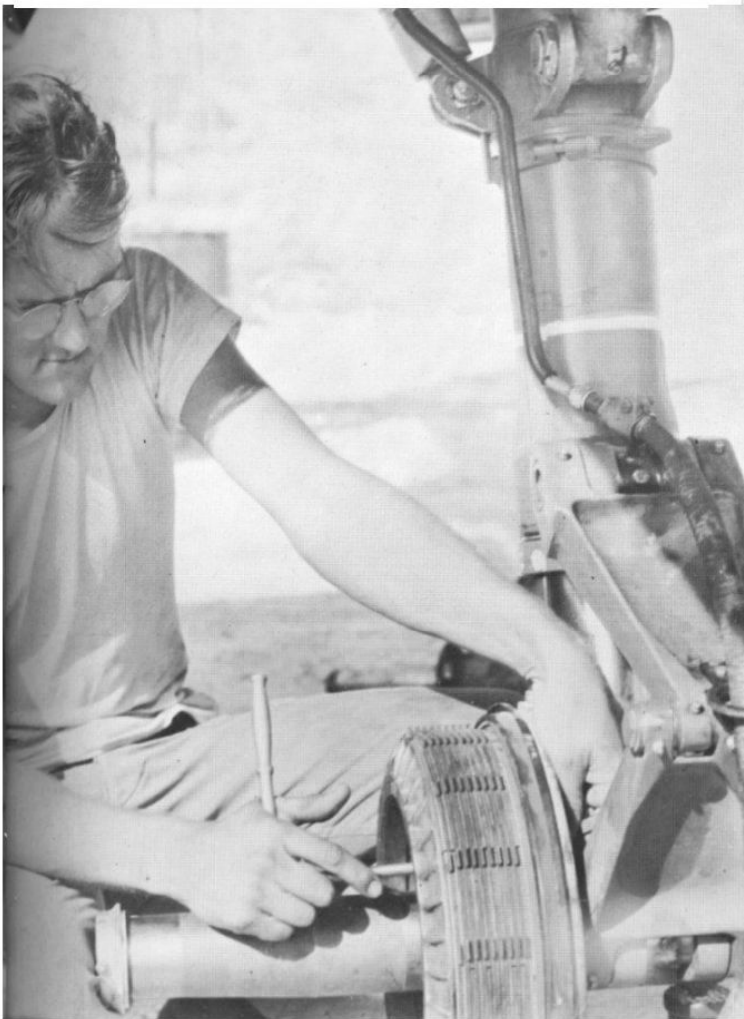
(Top) All the propeller work was done by Sgt. Kammerer and Cpl. Hachman. In the picture, they are working on the electrical contact points in the prop motor which change the pitch of the propeller to effect a constant engine RPM. (Bottom) Our only hydraulic specialist was Sgt. Coker. He is shown installing a multiple disc brake unit.
