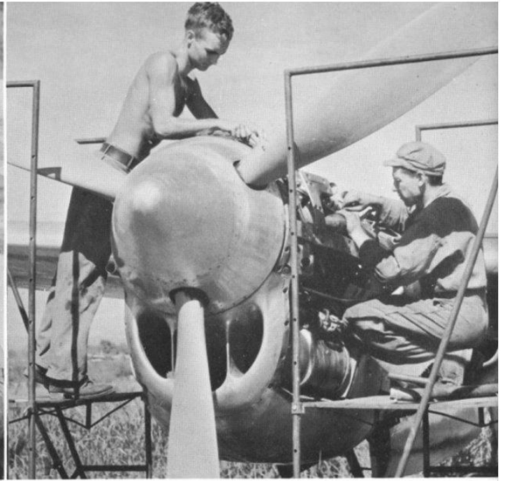
Sgts. Pflieger and Cope respectively check an oil thermostat and exhaust manifold.
